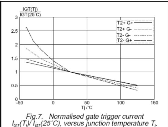
Fig.7. Normalised gate trigger current  $I_{GT}(T_j)/I_{GT}(25^\circ C)$ , versus junction temperature  $T_j$ .
