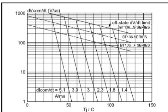
Fig.12. Typical commutation  $dV/dt$  versus junction temperature, parameter commutation  $dl/dt$ . The triac should commutate when the  $dV/dt$  is below the value on the appropriate curve for pre-commutation  $dl/dt$ .
