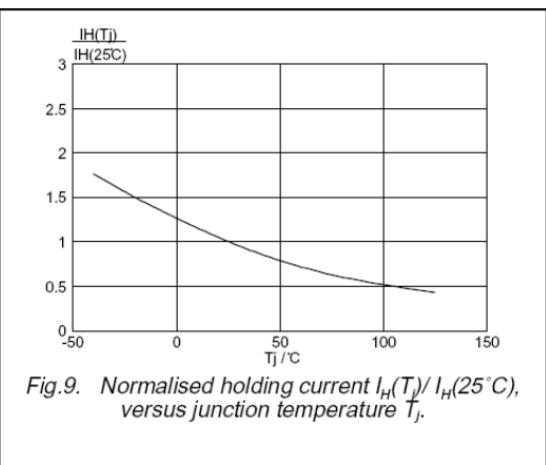
Fig.9. Normalised holding current  $I_H(T_j)/I_H(25^\circ C)$ , versus junction temperature  $T_j$ .
